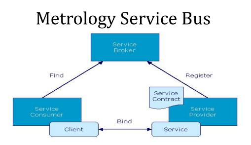
How it works is pretty simple. Both the Service Provider and the Service Consumer register with the Service Broker. The Service Provider will provide the Service Broker with a manifest of what service it offers, as well as its current state and location. And the Service Consumer registers itself with the Service Broker as well.
